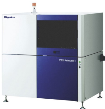
Rigaku ZSX Primus III+ high power, tube above, sequential WDXRF spectrometer
